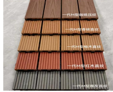
品名 (name): 户外塑木地板 (outdoor wpc floor) 规格 (size): 300mm宽 (width)*300mm长 (length)*20mm厚 (thick) 结构 (Structure): 实心-防滑槽 (Solid, one-sided anti-slip channel)
